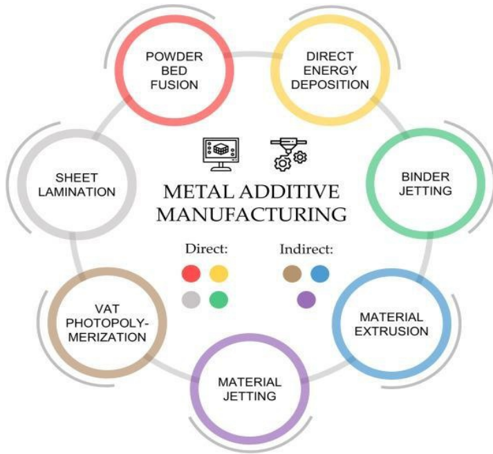
Figure 1. Classification of metal additive manufacturing processes according to ASTM standards. The figure classifies the major metal additive manufacturing technologies into direct and indirect processing routes based on how the final metallic component is produced. Source: [16]
