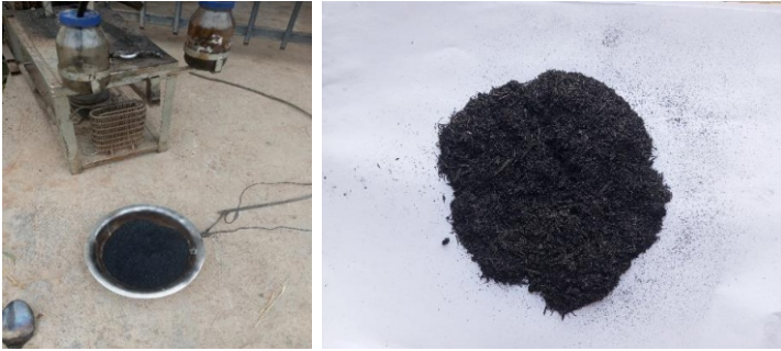
Figure 5: Rice husk (RHK) torrefied at 220°C for 30 minutes.
