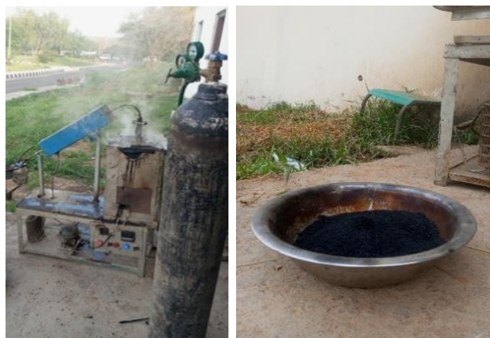
Figure 4: (a) Fixed-bed reactor and (b) torrefied coconut shell (CNS) obtained at 220 °C for 45 minutes
