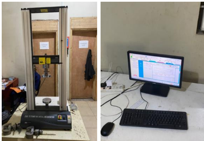
Figure 10: (a) Universal Testing Machine and (b) Computer interface and control system for data acquisition.
