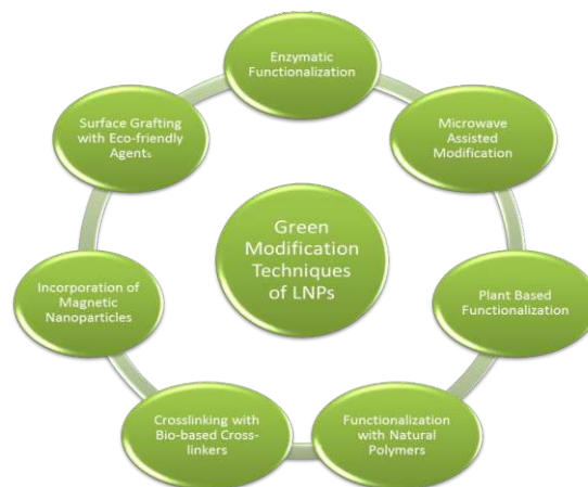
Fig 5: Green Modification of Lignin NPs
