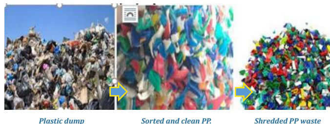
Plate 1: Waste plastics sorted from refuse into PP wastes and shredded for pyrolysis
